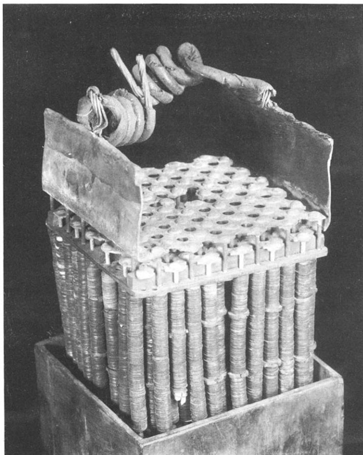
Fig. 2. Early tubular battery construction, about 1900. The tubes are formed of hard rubber washers, piled upon another. (Courtesy ESB Inc., Philadelphia)
